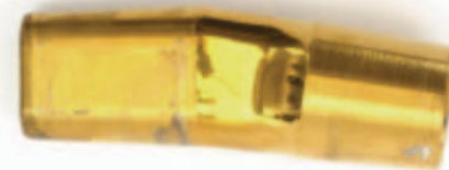
Fig. 8: Representative photograph of the surfaces of the neck post fatigue – specimen 1.1
