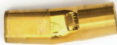
Fig. 8: Representative photograph of the surfaces of the neck post fatigue – specimen 1.1
