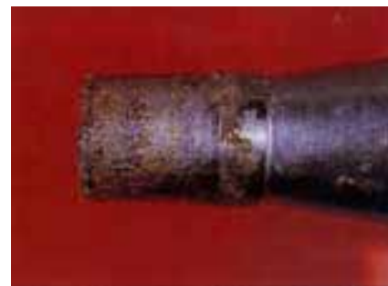
Corrosion on Co-Cr/Co-Cr taper 10 yrs postop
