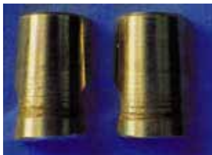
Fretting marks on Ti-6Al-4V taper 4 yrs postop
