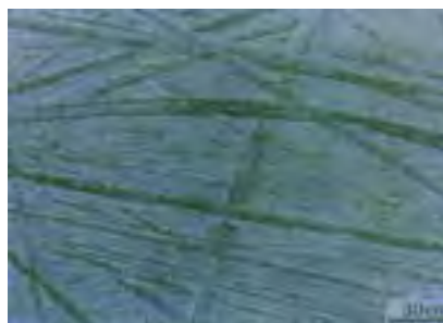
Scratches in polyethylene liner from abrasive third-body wear
