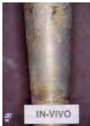
Small areas of fretting on modular stem taper 6 yrs postop
