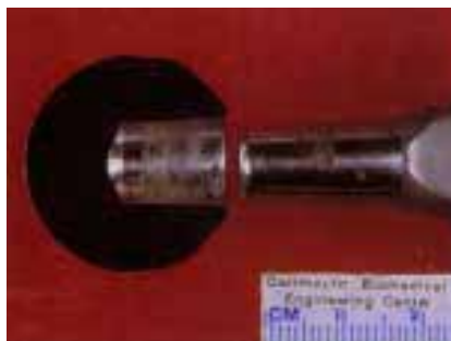
Corrosion on mixed-metal taper 22 months postop
