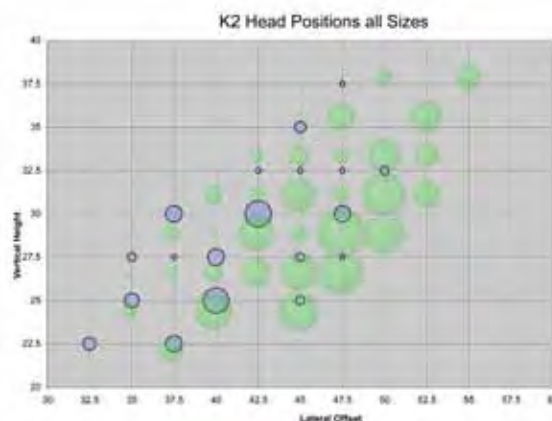
Green previous Apex modular straight stem design Blue tapered K2 stem design
