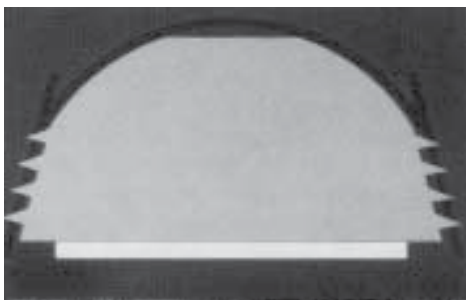
Figure 15 Hemispherical shell with conical threads.
